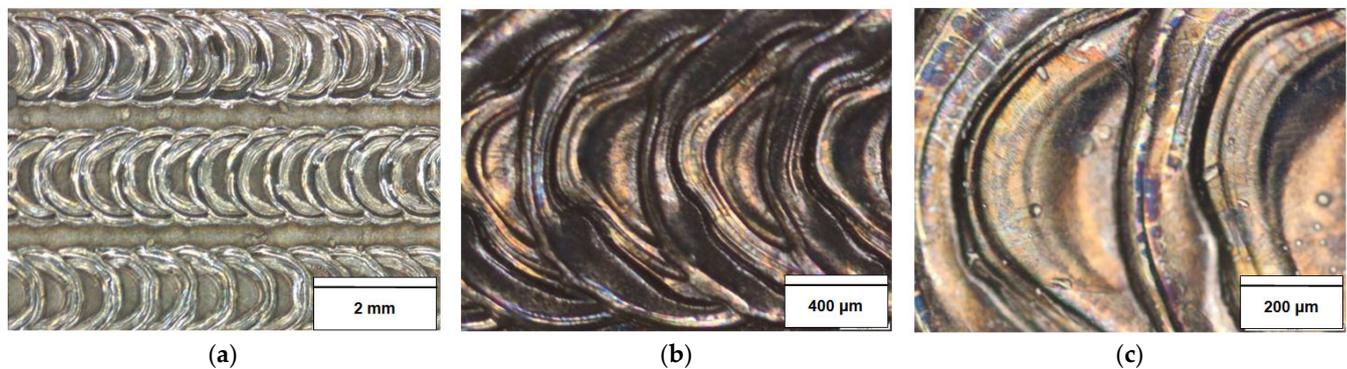
**Figure 10.** Etched and blackened AISI 316L surface subjected to laser texturing of 2500 W laser beam power with pulse focus of 0.5 mm and frequency of 3 Hz: (a) 10× magnification by ZEISS; (b) 50× magnification by Olympus; and (c) 100× magnification by Olympus.
