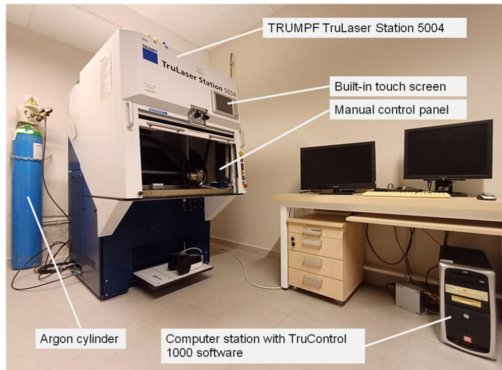
**Figure 1.** Nd: YAG TRUMPF TruLaser Station 5004 experimental setup.
