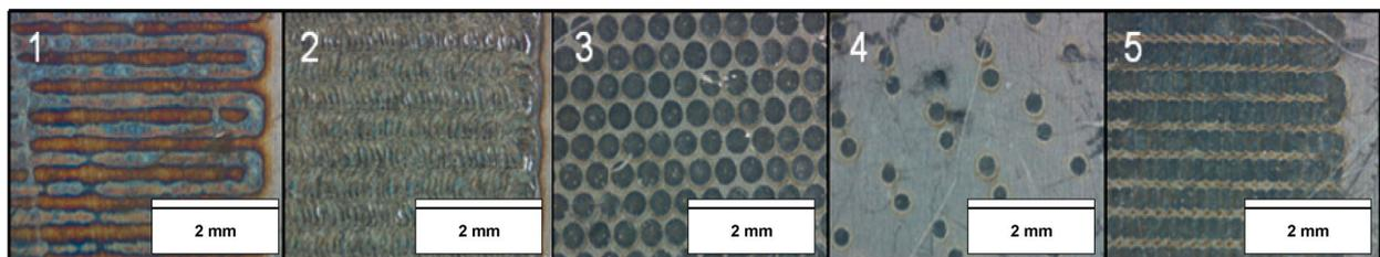
**Figure 2.** Paths obtained by laser surface layer modifications performed on AISI 316L steel.
