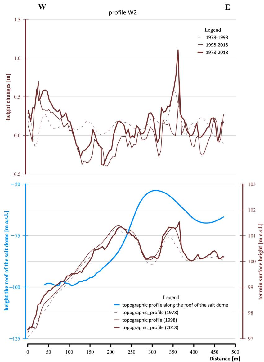
**Figure 10.** The topographical profiles of the ground surface in the particular years with the profile line of the top surface of the salt deposit. The plot at the top shows the height changes along the W2 profile line in the analyzed time intervals.
