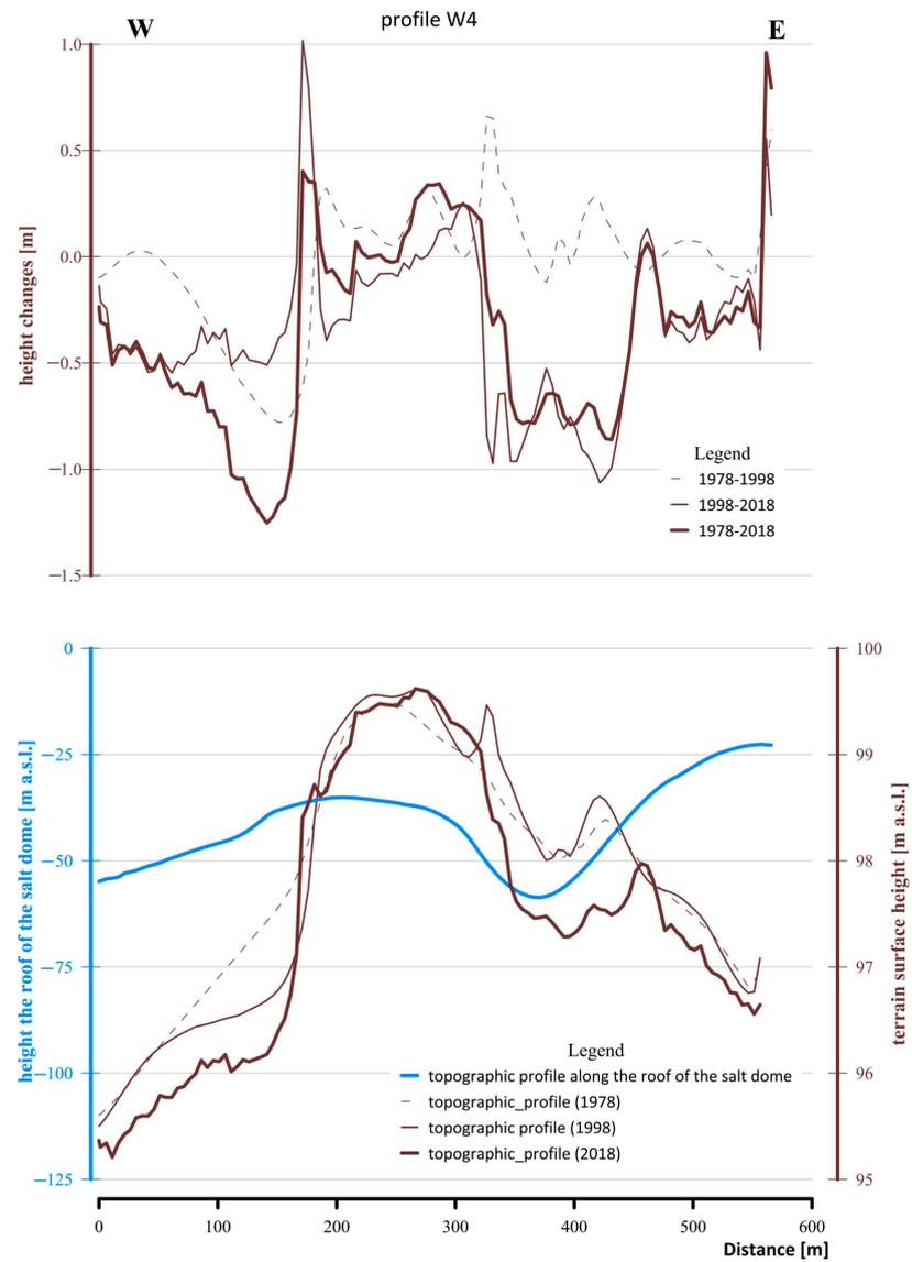
**Figure 12.** The topographical profiles of the ground surface in the particular years with the profile line of the top surface of the salt deposit. The plot at the top shows the height changes along the W4 profile line in the analyzed time intervals.
