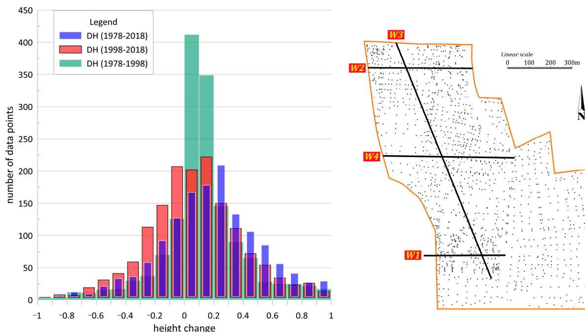
**Figure 8.** Histogram of height changes of points (in meters) for the assumed time intervals and the location of reference points (from 1978) on the right.
