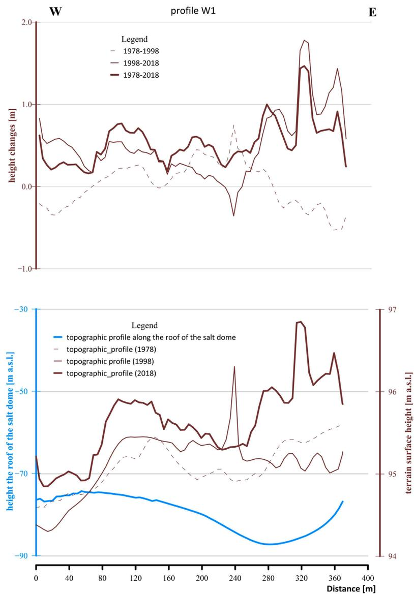
**Figure 9.** The topographical profiles of the ground surface in the particular years with the profile line of the top surface of the salt deposit. The plot at the top shows the height changes along the W1 profile line in the analyzed time intervals.
