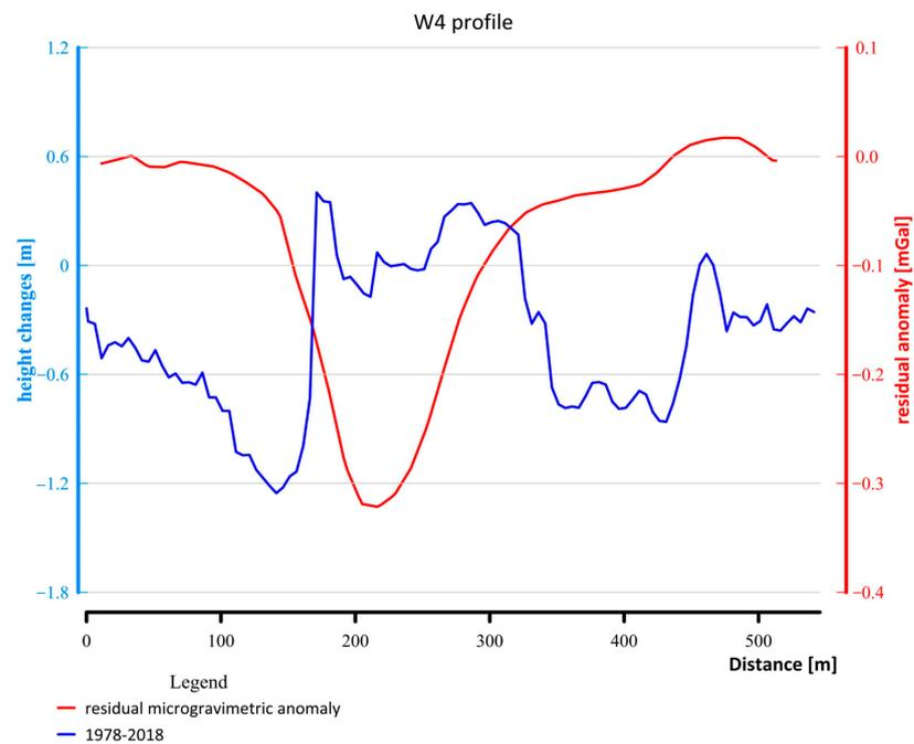
**Figure 13.** The distribution of residual microgravity anomaly (red line) and height changes between 1978 and 2018 along the W4 profile line (blue line).
