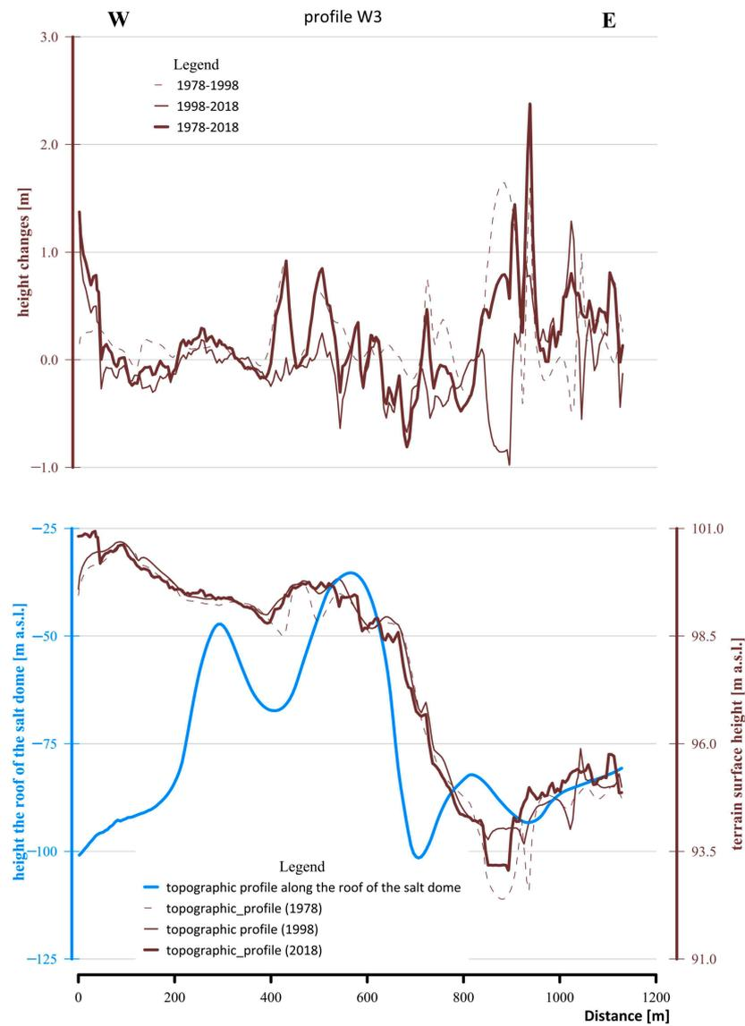
**Figure 11.** The topographical profiles of the ground surface in the particular years with the profile line of the top surface of the salt deposit. The plot at the top shows the height changes along the W3 profile line in the analyzed time intervals.
