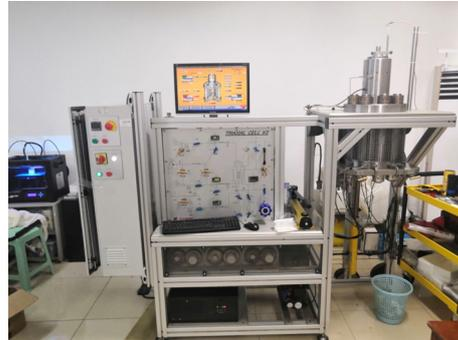
**Figure 1.** The fully automatic triaxial servo system for rocks.
