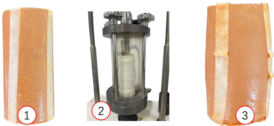
Figure 3. Triaxial test sample and test process (1. triaxial sample; 2. sample being sheared; and 3. shear damage of the sample).
