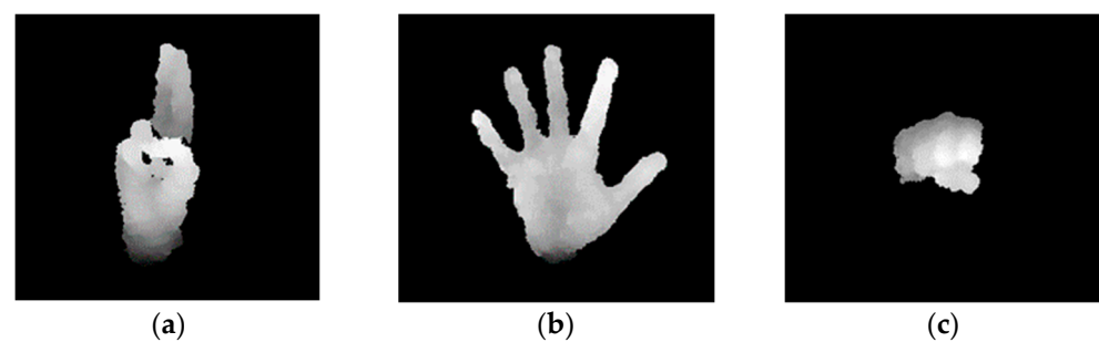
Figure 1. Hand gesture modes for imitating computer mouse behavior: (a) mode 1, (b) mode 2, and (c) mode 3.
