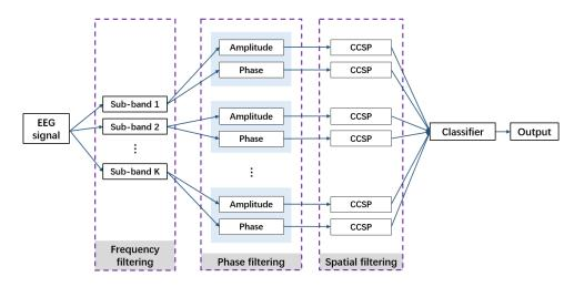
Figure 1. Architecture of the proposed MDCCSP.
