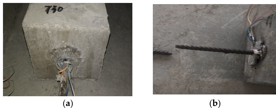
Figure 8. Failure modes of the specimens. (a) Pull-out failure of steel bar; (b) tensile failure of steel bar.
