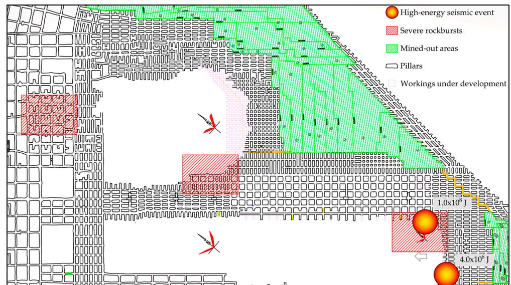
Figure 2. Example of room-and-pillar mining with roof deflection in Polish copper mines—the site where the proposed approach was validated.
