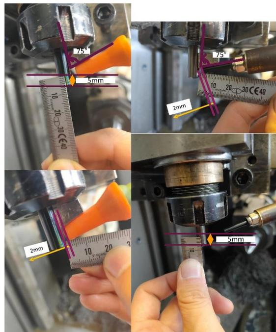
**Figure 2.** Nozzle position for tribological tests.
