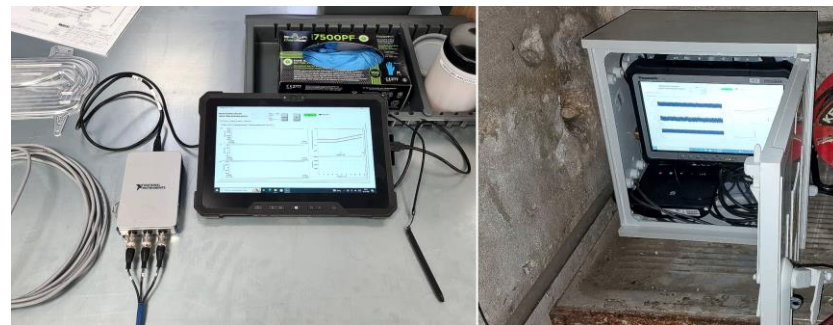
Figure 5. View of the card and the computer unit before and after mounting in the housing.
