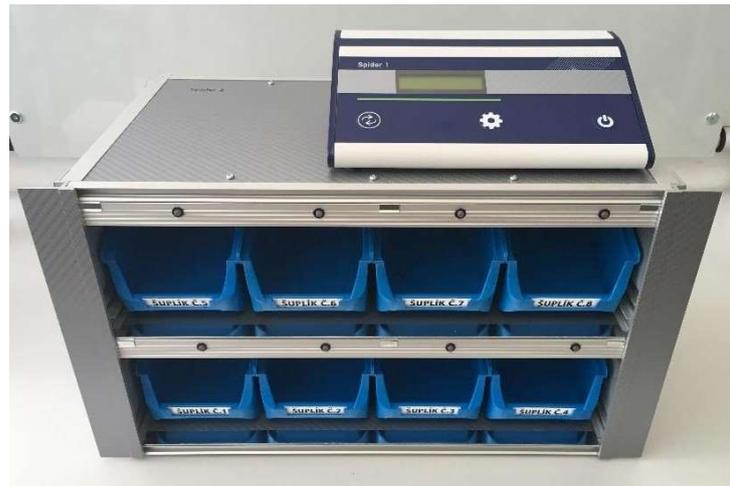
**Figure 4.** Constructed Pick-to-Light device labelled Spider 1.
