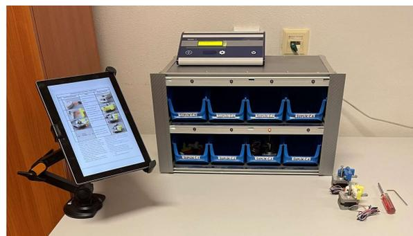
**Figure 7.** Assembly workplace with PTL.
