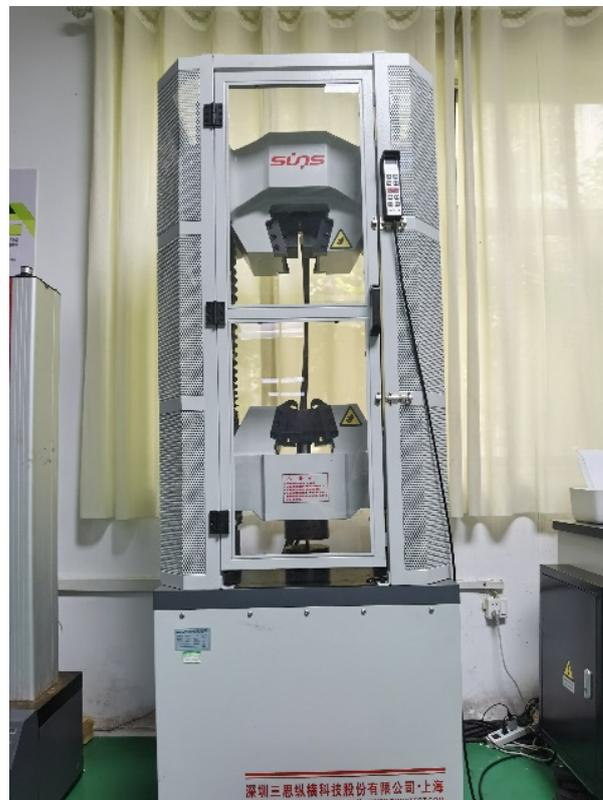
**Figure 5.** WAW-600D electro-hydraulic servo universal tensile testing machine.
