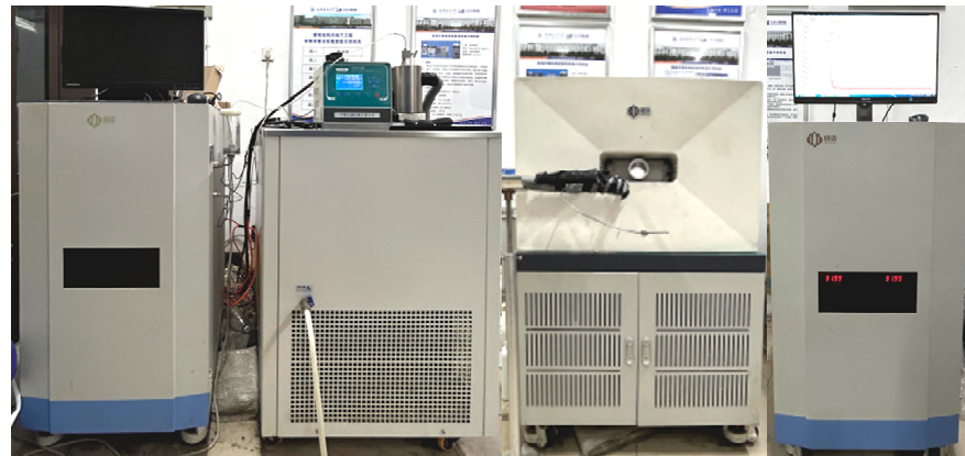
Figure 14. Low-temperature and high-pressure nuclear magnetic resonance test platform.
