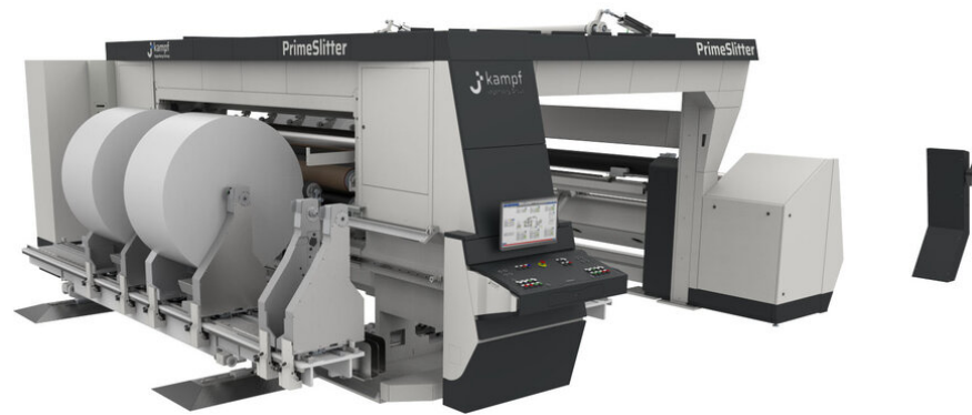
Figure 3. Visualization of the slitting machine that was used to generate the data for the experiments. The image is provided by 'Kampf Schneid- und Wickeltechnik GmbH & Co. KG', Wiehl, Germany.
