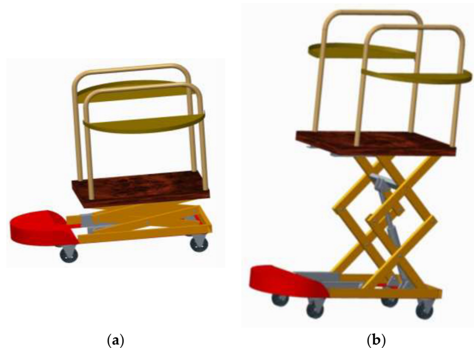
Figure 1. Positions of the base of the scissor mechanism (a) in the folded state and (b) in the maximum raised state.
