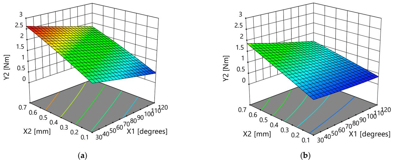
Figure 9. The influence of the drill tip angle and tooth bite on the thrust force: (a) flat drill (a,b) helical drill.
