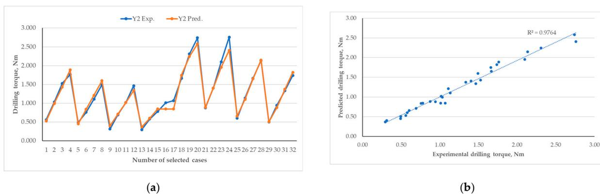
**Figure 7.** The graphical comparison between the experimental and predicted values of drilling torque: line chart (a) and scatter plot (b).
