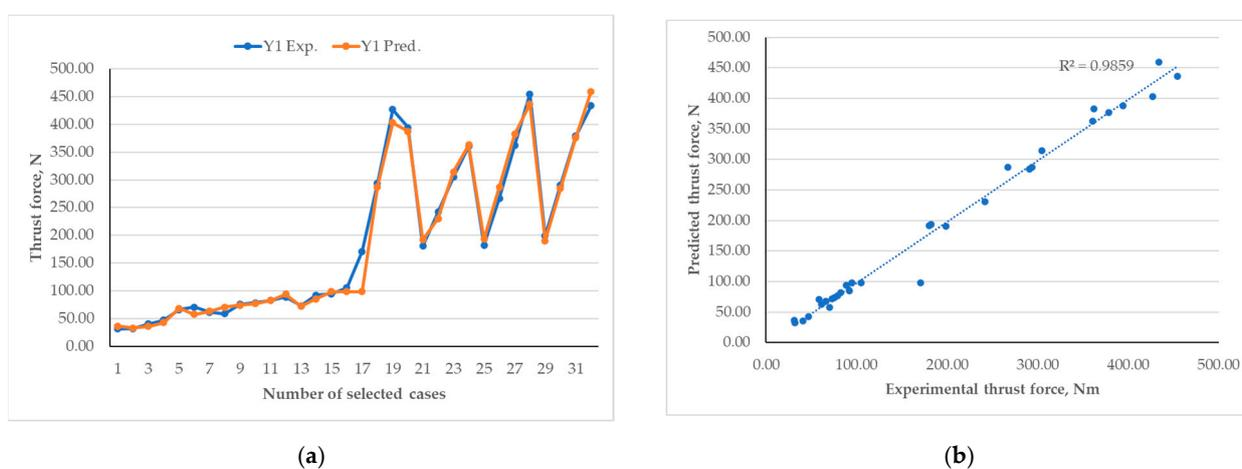
**Figure 6.** The graphical comparison between the experimental and predicted values of thrust force: linechart (a) and scatter plot (b).
