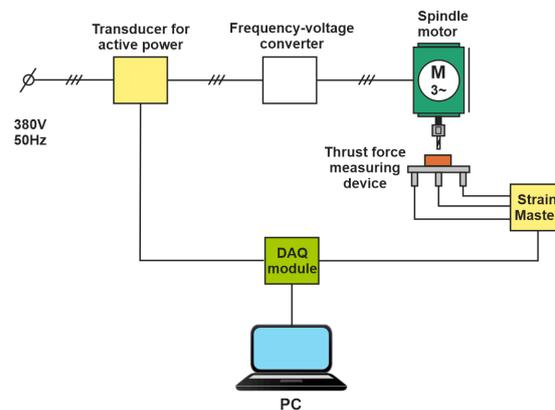
**Figure 3.** Connection diagram of the equipment for measuring the dynamic parameters of the drill.
