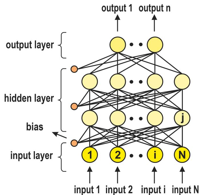
**Figure 4.** The multi-layer perceptron architecture.
