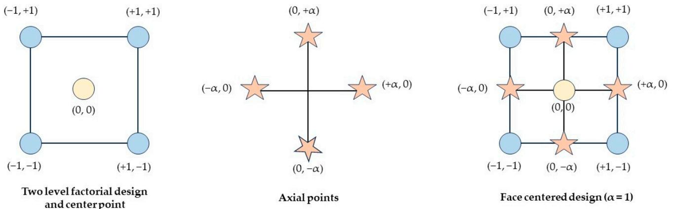
Figure 5. The structure of a face centered composite design.
