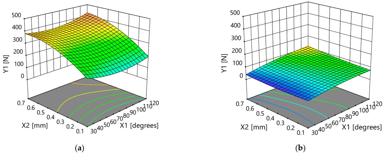
**Figure 8.** The influence of the drill tip angle and tooth bite on the thrust force: flat drill (a) and helical drill (b).
