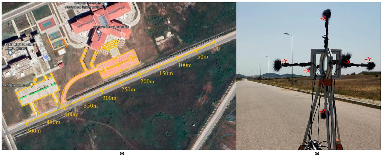
**Figure 14.** (a) Experiment site for explosion sound recording (b) microphone array and axes used.
