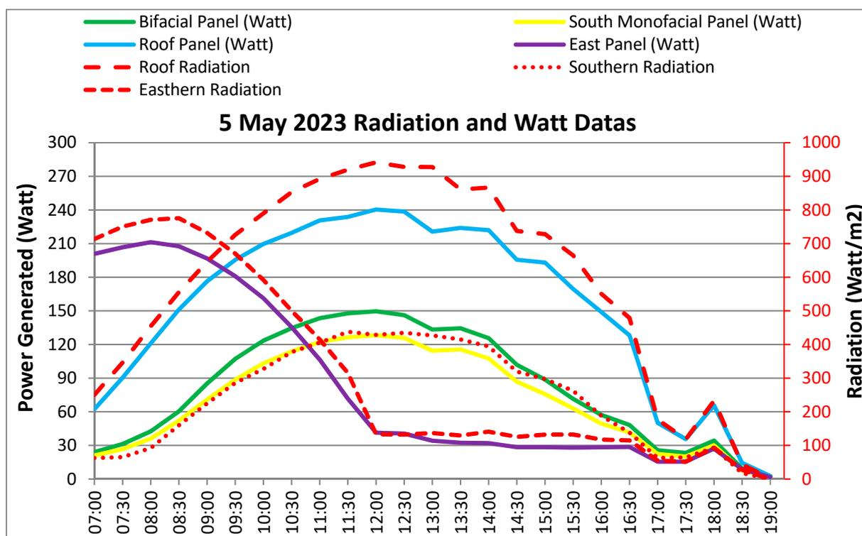
Figure 4. Power and radiation data produced by the experimental setup on 5 May 2023.
