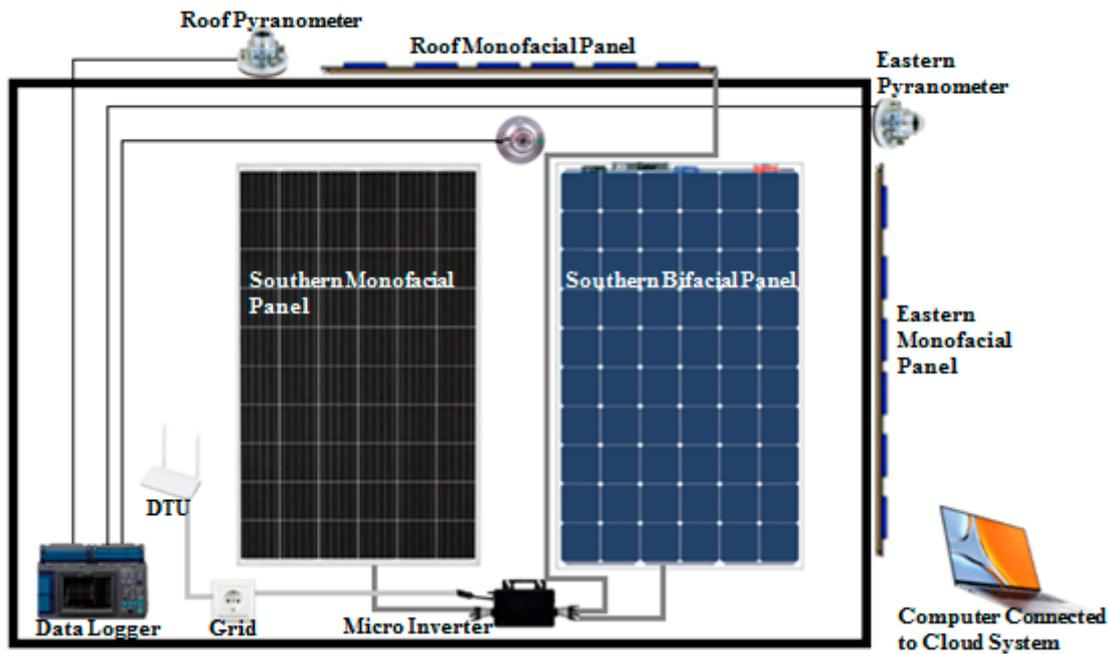
**Figure 2.** Measurement instruments and schematic representation of the experimental setup.
