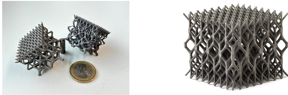
**Figure 13.** Additively manufactured lattice cubes with topology and radii gradients that are constructed using the discussed method.
