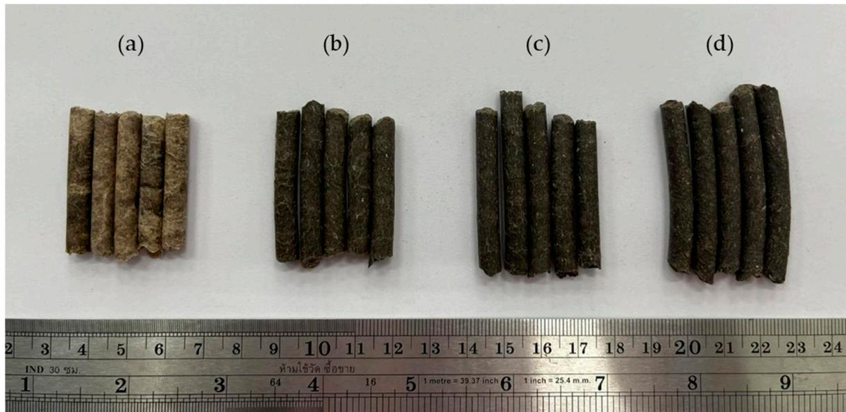
**Figure 1.** The completely randomized samples of each condition manufactured with sawdust/RDF ratios, (a) 100/0, (b) 50/50, (c) 60/40, and (d) 70/30.
