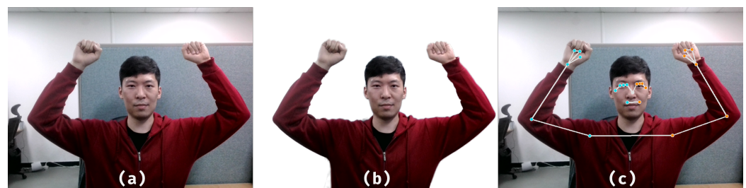
Figure 2. Results of RVM and MediaPipe Pose. (a) Original input frame of the upper body in 640 \times 480 resolution. (b) RVM output without background. (c) Upper-body joints from MediaPipe Pose.
