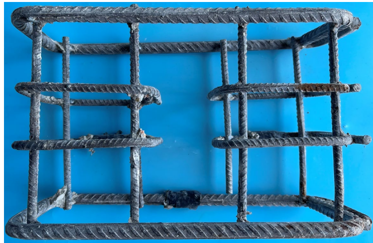
Figure 16. Stirrup skeleton after the test.
