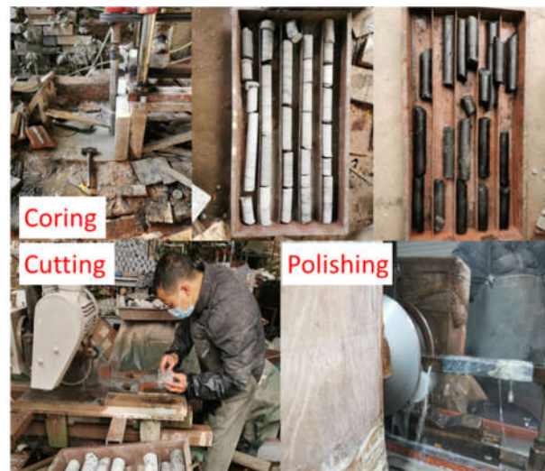
Figure 4. Processing of standard specimens.
