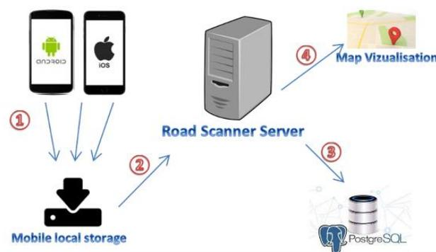
**Figure 2.** Solution Architecture. The sequence from 1 to 4 represents the time order of the data flow from collection to map visualization.
