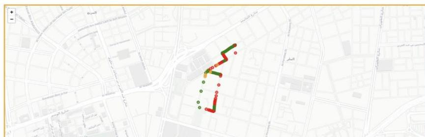
**Figure 5.** Map visualization with playback features. The circles represent samples of recording while their colors represent their corresponding labels (“Potholed”, “Bumps”, “Smooth”, and “Other”).
