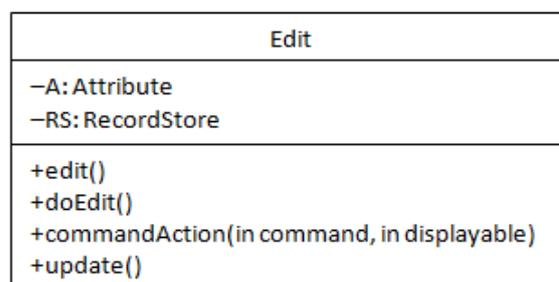
Figure 2. One-function structure for Edit [40].
