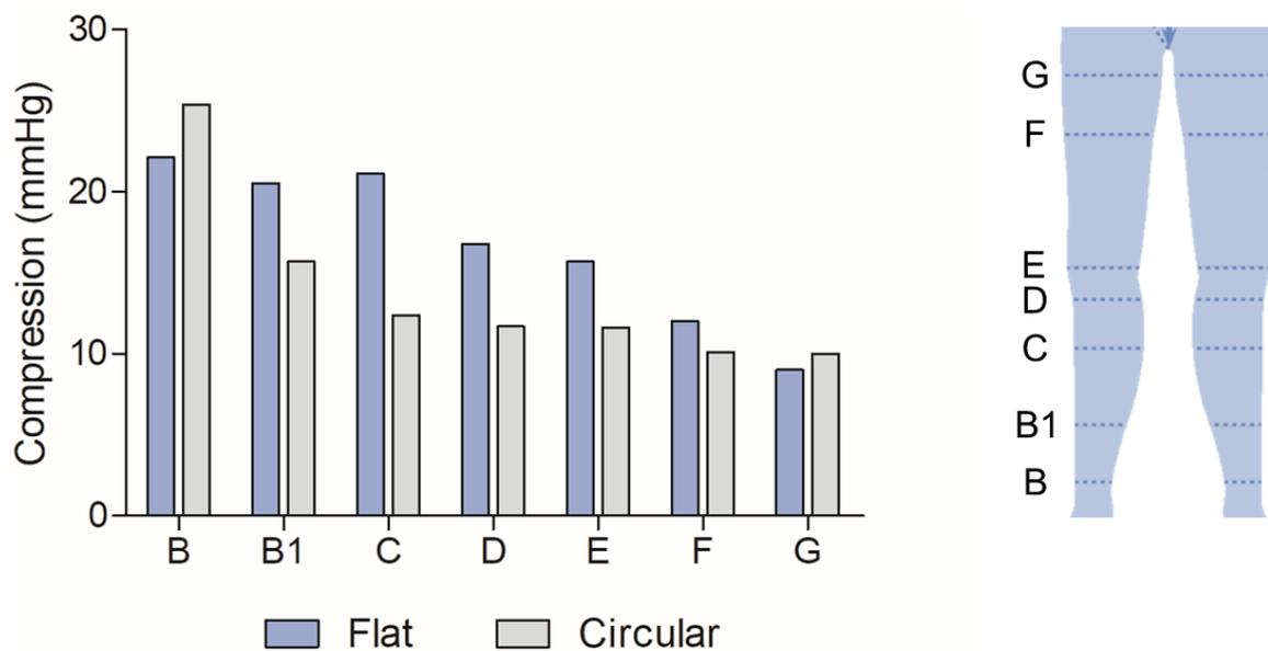
**Figure 3.** Average compression values of the prototypes measured in the system MST MK V, Swiss-lastic Ag St, Gallen, Swiss. Reference points of each measurement point extracted from [12].
