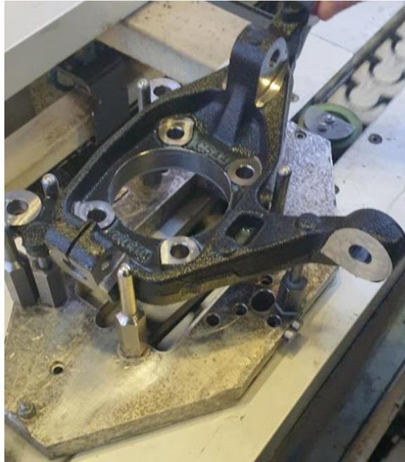
**Figure 4.** Car steering knuckle with machined surfaces for tool wear testing.
