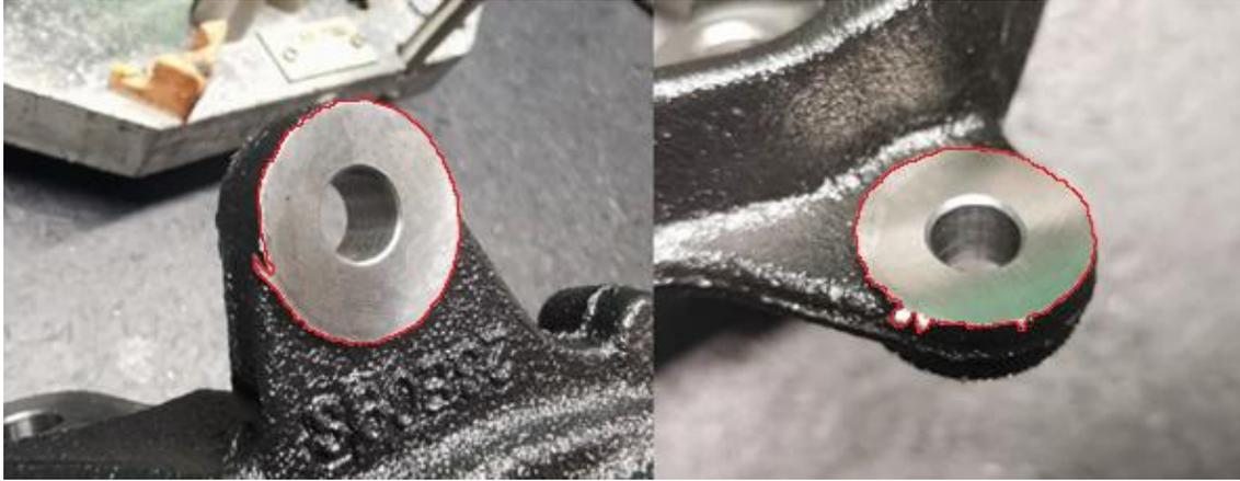
**Figure 6.** Detailed photos taken with a service life of 170–200 tool cycles.
