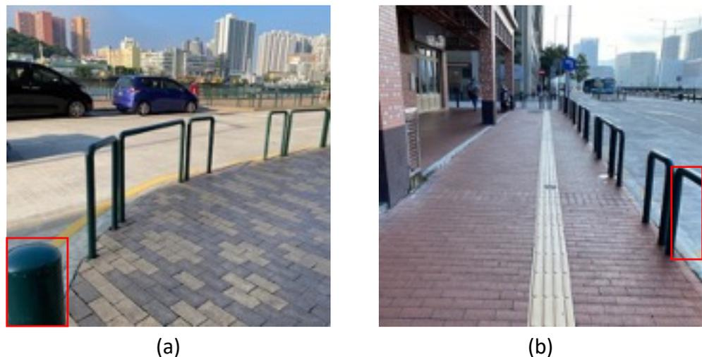
**Figure 8.** Example of partially out-of-view objects. (a) Only the upper part of the pillar was detected. The system could not estimate its distance; (b) only half of the fence was detected. The POI indicated by the bounding box is far from the closest point of the object. Both cases introduce errors into the system.
