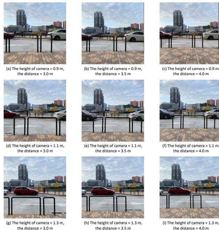
Figure 6. Experiments for acquiring the camera’s focal length.
