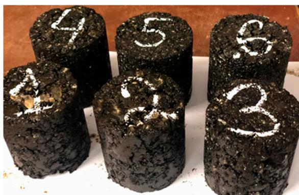
**Figure 1.** Samples of asphalt concrete mix.
