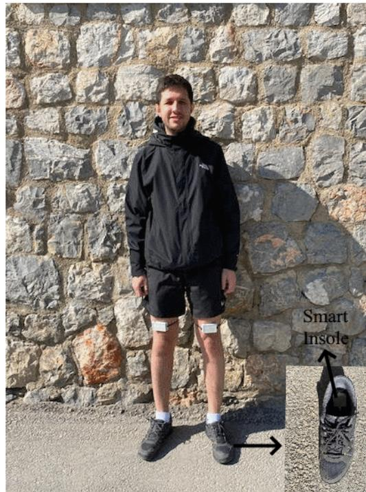
**Figure 3.** Sensor position on the human body.
