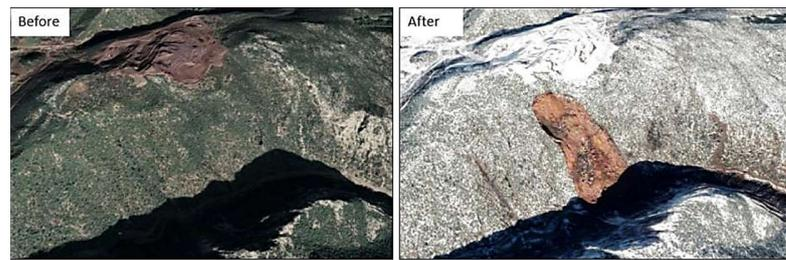
**Figure 5.** Comparison of a landslide before (**left**) and after (**right**) the earthquake, showing the movement and deposition of soil and rocks on a slope. The images were obtained from Google Earth Pro, with the lat long coordinates of 37°00' N, 36°35' E and the date of 27 December 2022 (before) and 7 February 2023.
