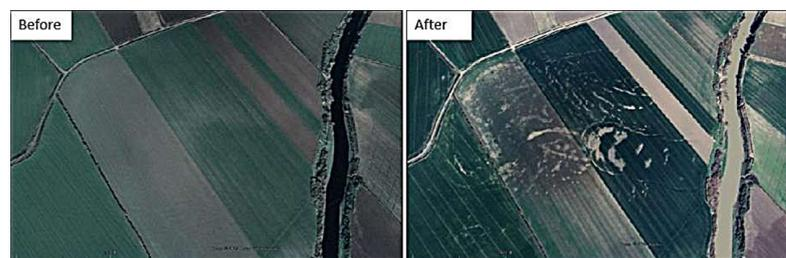
**Figure 6.** Comparison of site liquefaction before (**left**) and after (**right**) the earthquake, showing the formation and expulsion of water and sand on a flat area. The images were obtained from Google Earth Pro, with the lat long coordinates of 36°15' N, 36°14' E and the date of 22 December 2022 (before) and 14 February 2023.
