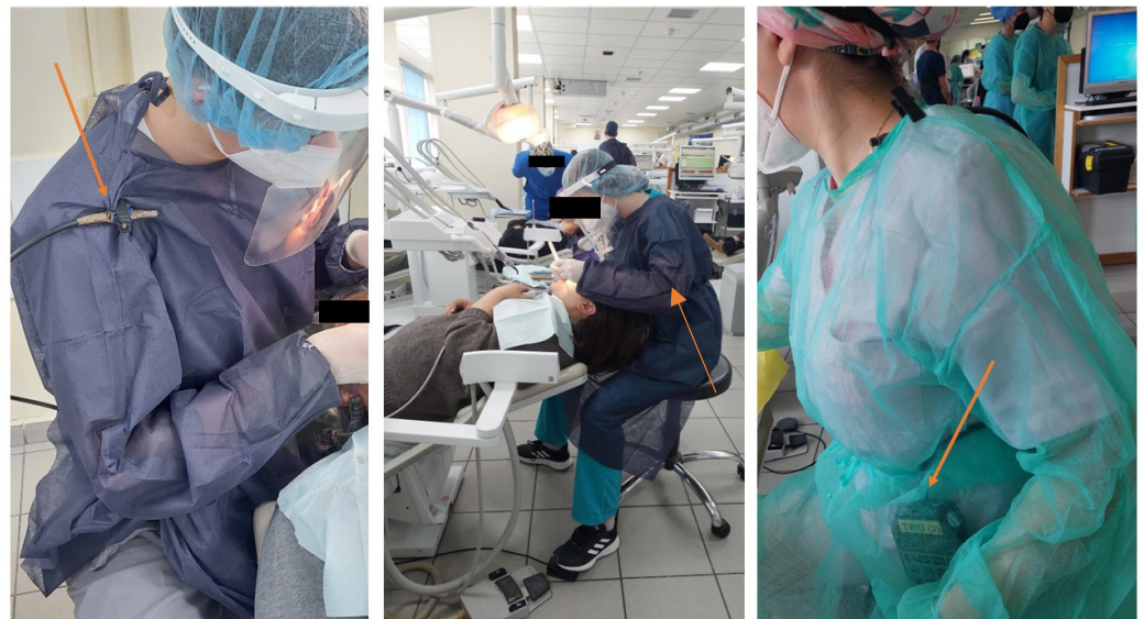
Figure 2. Students wearing personal sound measurement equipment (arrows show position of atomic measurement equipment).
