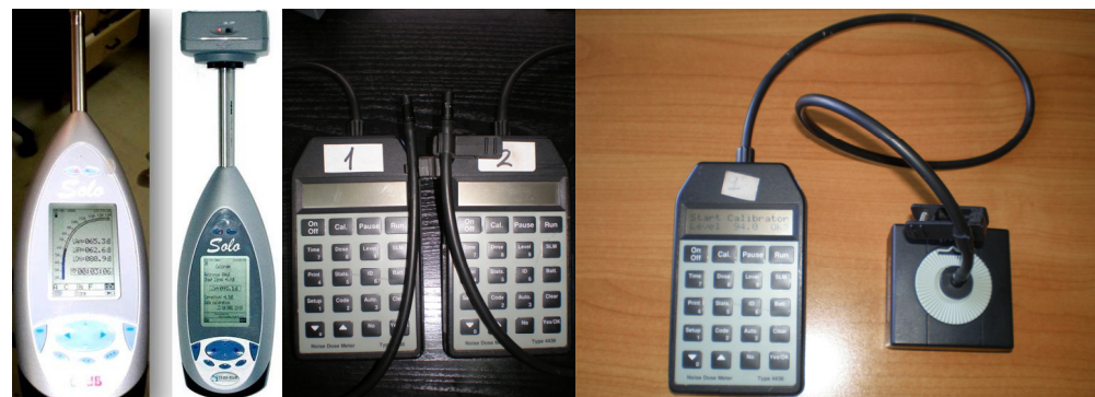
Figure 3. The Solo 01 dB-Metravib and the two Brüel and Kjær Noise Dose Meters (Type 4436) were calibrated prior to testing noise measurements.
