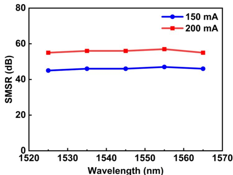
Figure 6. The side mode suppression ratio (SMSR) versus tuning wavelength at injection currents of 150 mA and 200 mA, respectively.
