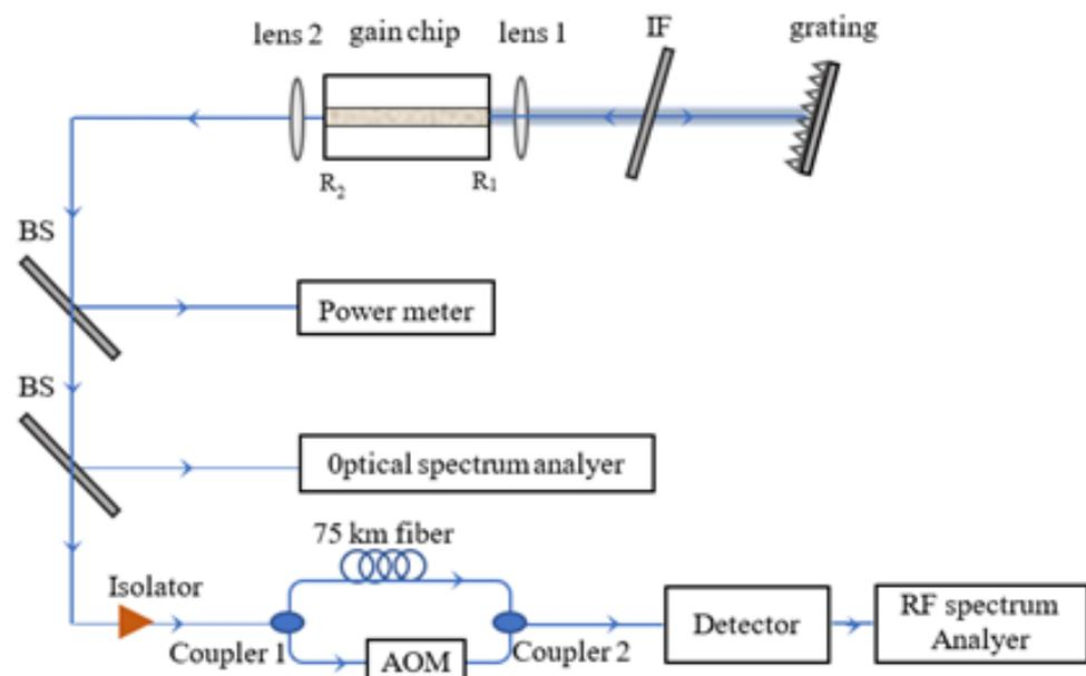
**Figure 1.** Experimental scheme of the external cavity diode laser is shown. The external cavity is composed of the lens, interference filter and diffraction grating. The laser is output from  $R_2$  and coupled into a fiber to measure the power, optical spectrum and linewidth.
