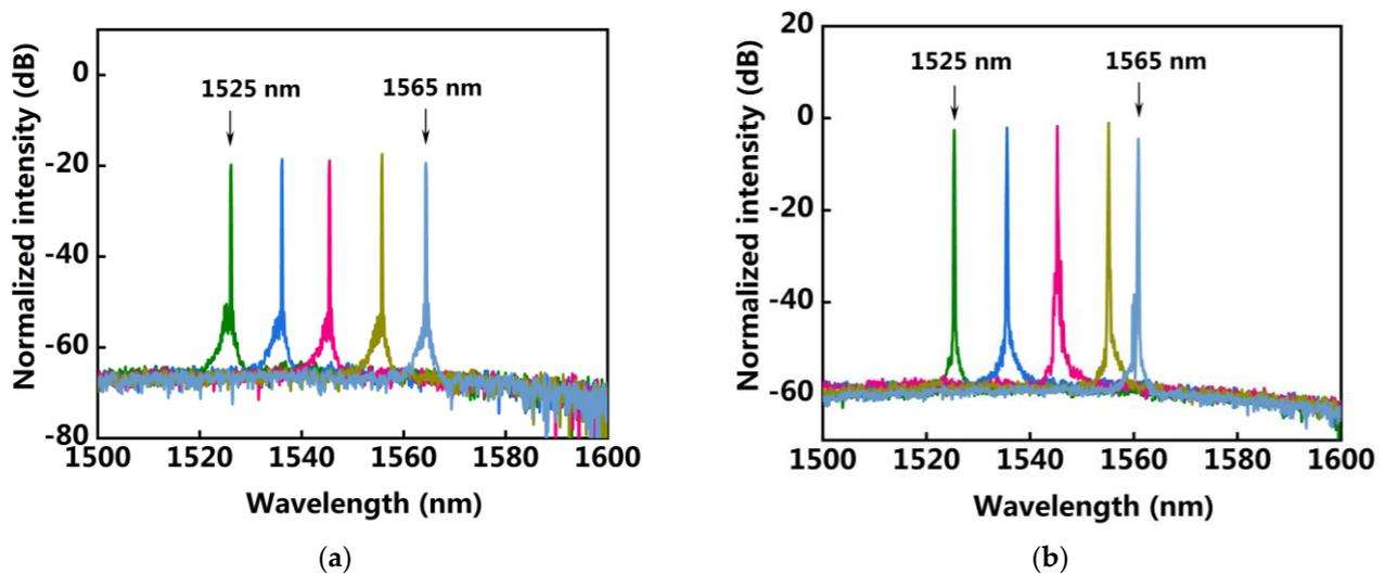
**Figure 2.** Optical spectra of the output beam for the ECDLs with (a) an injection current of 150 mA and (b) an injection current of 200 mA. The tunable range is both 40 nm from 1525 nm to 1565 nm. The peaks in the tuning range correspond to different grating positions.
