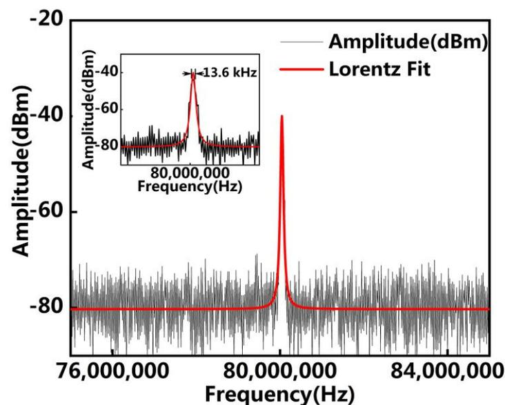
**Figure 3.** The linewidth spectrum at a wavelength of 1555 nm is 13.6 kHz.
