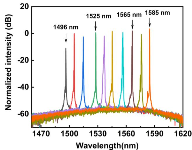
**Figure 4.** The optical spectra without an interference filter are measured with an injection current of 200 mA. The peaks correspond to different grating positions over the tuning range.
