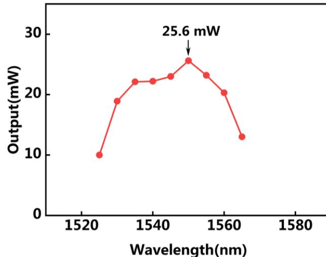
Figure 7. The output power as a function of wavelength with an injection current of 200 mA.
