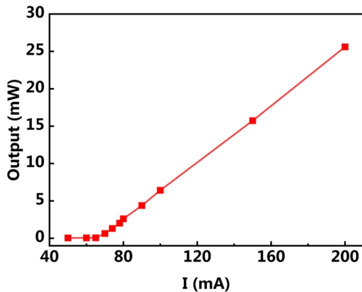
Figure 5. The threshold current at a wavelength of 1550 nm is measured.
