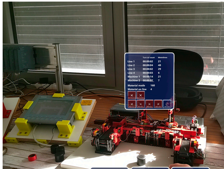
Figure 20. Production line detection in reality.
