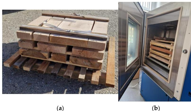
**Figure 1.** Mini-stacks of 50 mm thick Turkey oak lumber prepared for air-drying (a) and for kiln-drying in a KPK200 climate chamber (b).
