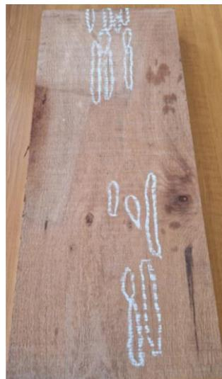
**Figure 7.** Surface cracks after the steaming of Turkey oak boards.
