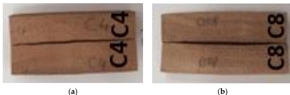
**Figure 12.** Case-hardening samples of kiln-dried 50 mm thick Turkey oak lumber: (a) steamed board (gap opening = 2 mm) and (b) unsteamed board (gap opening = 3 mm).
