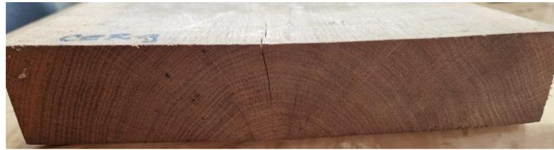
Figure 9. End cracks in air-dried 50 mm thick Turkey oak lumber despite paraffin-based end protection.
