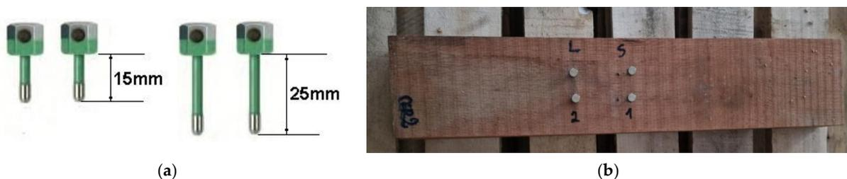
**Figure 4.** Monitorization of the moisture content of wood during kiln-drying by two pairs of V2A sensors, of different lengths (a), in order to measure separately the core and surface MC of the board (b).
