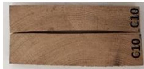
Figure 10. Case-hardening sample of air-dried 50 mm thick Turkey oak lumber (gap opening = 2.5 mm).
