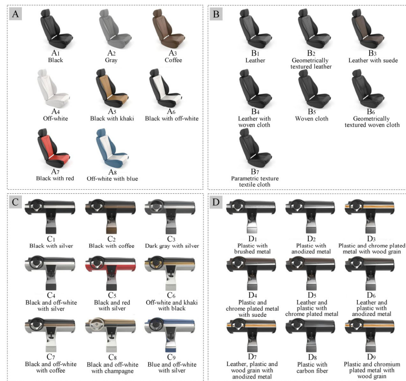
Figure 5. The interior CMF samples for examination: (A) the seat color group, (B) the seat material group, (C) the bridge color group and (D) the bridge material group.
