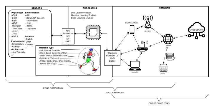
Figure 6. Layered Structure of Wearable Computing.
