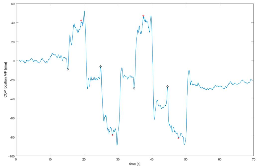
Figure 4. Exemplary COP displacements registered during measurement with use of VR and scenery oscillations at 0.2 Hz. Black rhomboids represent points of leaning start, red stars are points of registered maximums during leaning.
