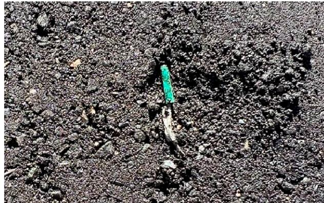
**Figure 5.** Temperature sensor in the first lift of the binder course.
