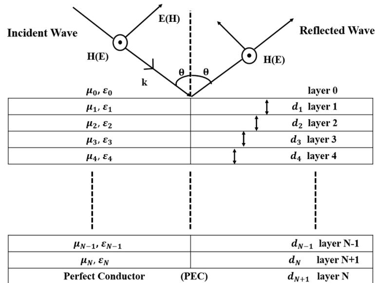
Figure 1. Illustration of the microwave absorber structure.
