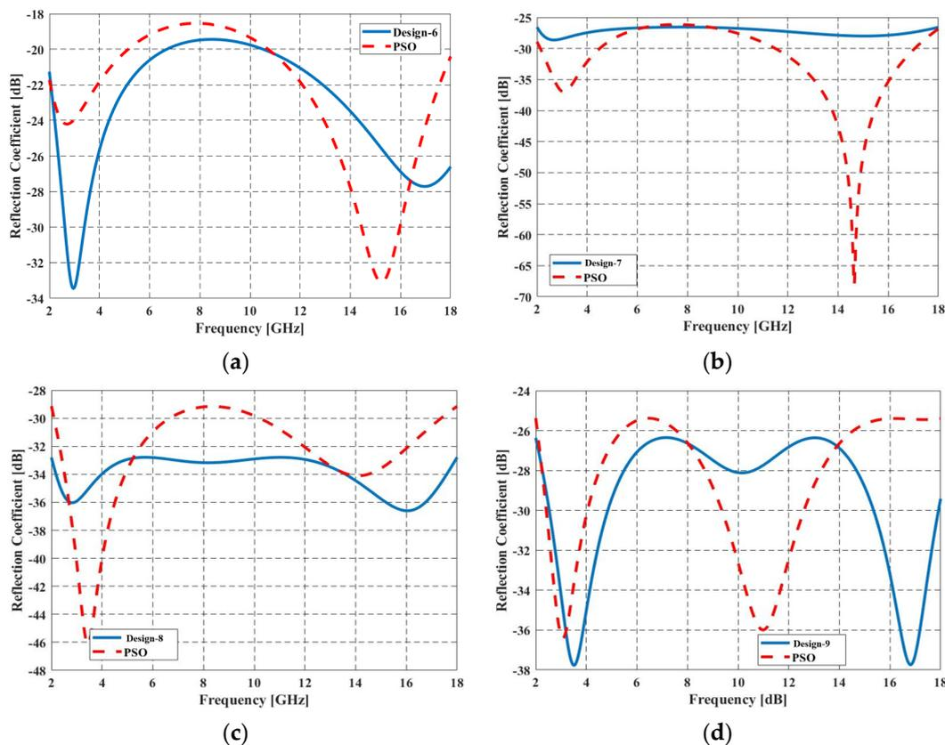
**Figure 10.** RC of 5-layer MAs optimized for 2–18 GHz FR for TM polarization for (a) 30° (Design-6), (b) 45° (Design-7), (c) 60° (Design-8), and (d) 75° (Design-9) angles of incidence.
