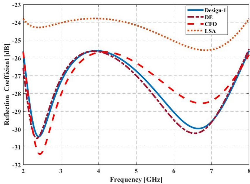
Figure 5. RC of 5-layer absorber optimized for 2–8 GHz FR for normal incidence (Design-1).
