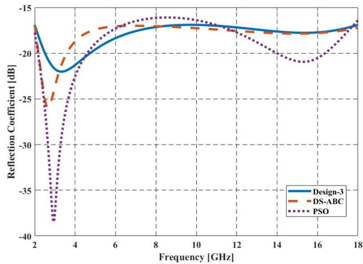
Figure 7. RC of 5-layer absorber optimized for 2–18 GHz FR for normal incidence (Design-3).
