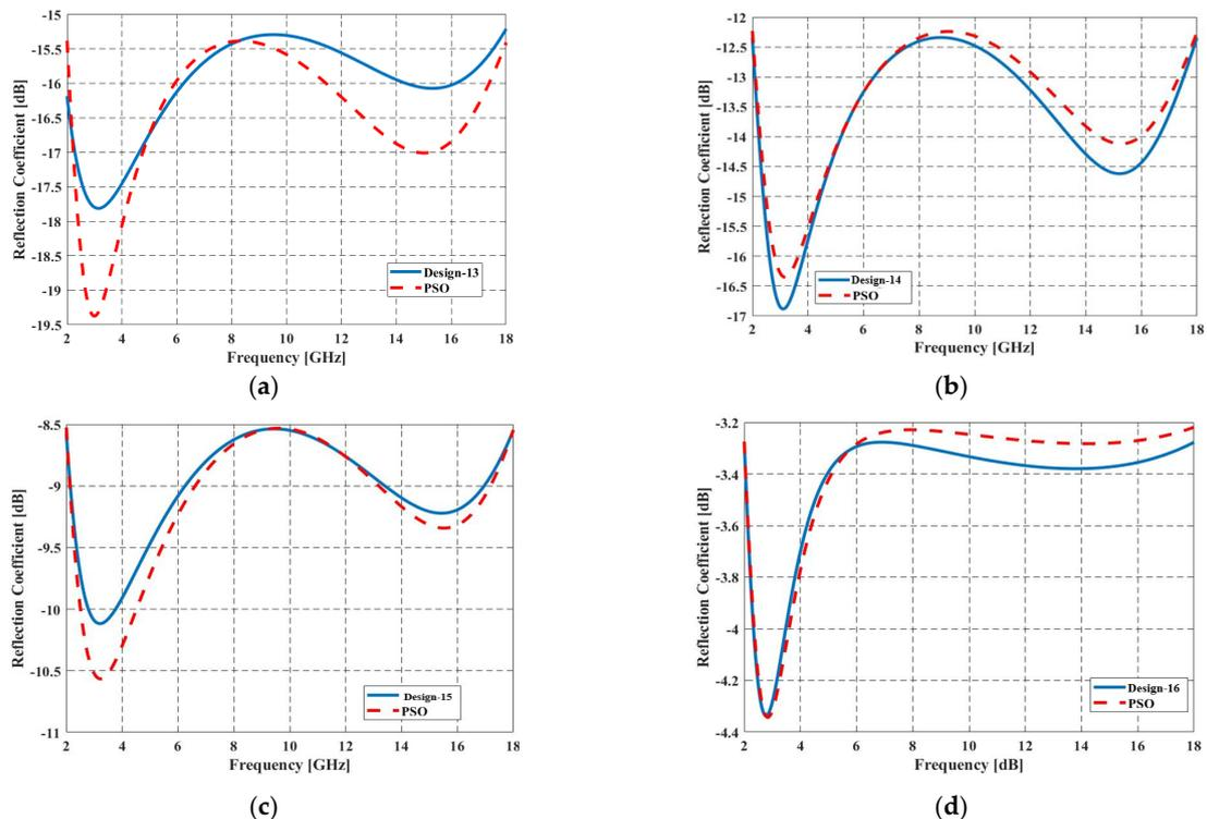
**Figure 12.** RC of 5-layer absorber optimized for 2–18 GHz FR for TE polarization for (a) 30° (Design-13), (b) 45° (Design-14), (c) 60° (Design-15), and (d) 75° (Design-16) angles of incidence.
