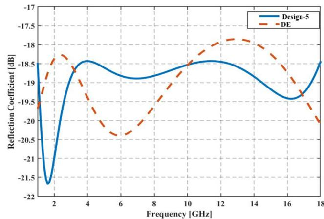
**Figure 9.** RC versus frequency of 7-layer MA for 1–18 GHz FR (Design-5).
