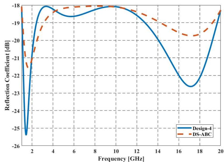
Figure 8. RC of 5-layer absorber optimized for 1–20 GHz FR for normal incidence (Design-4).
