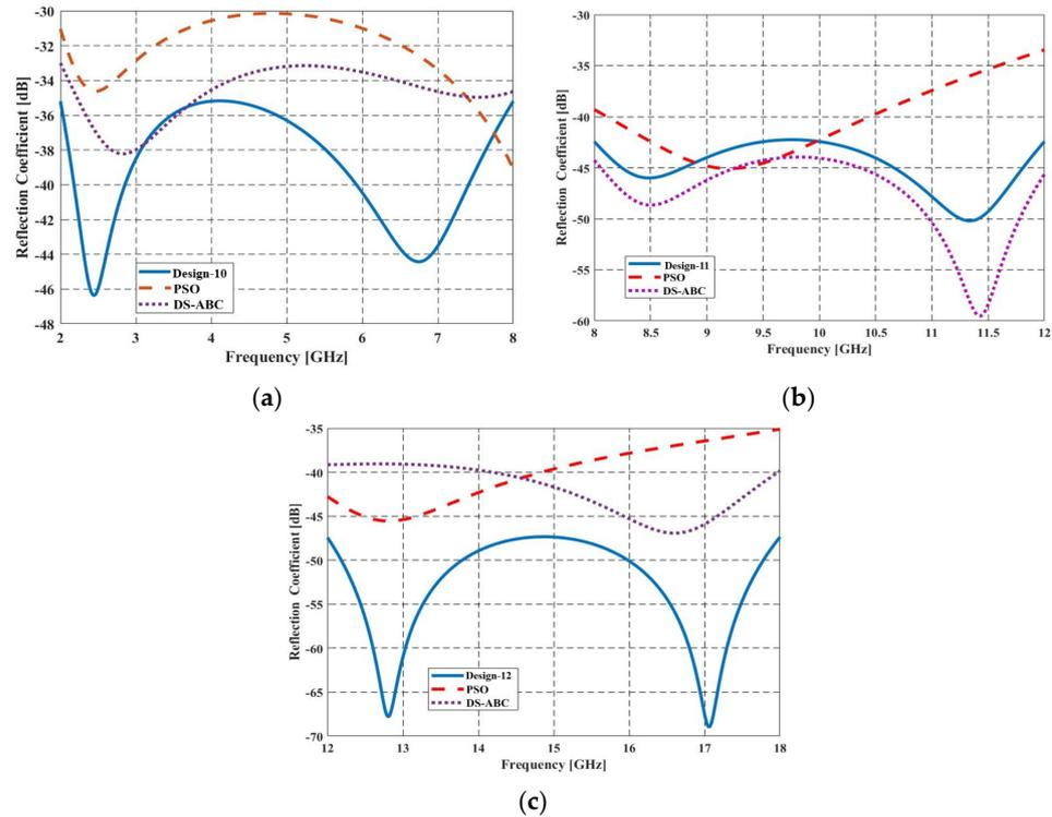
**Figure 11.** RC of 5-layer MAs optimized for (a) 2–8 GHz, (b) 8–12 GHz, and (c) 12–18 GHz FRs for TM polarization for  $45^\circ$  angle of incidence.
