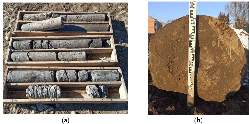
Figure 5. (a) The cores drilled from the finished column (in the ground). (b) Measured diameter of DSM column.
