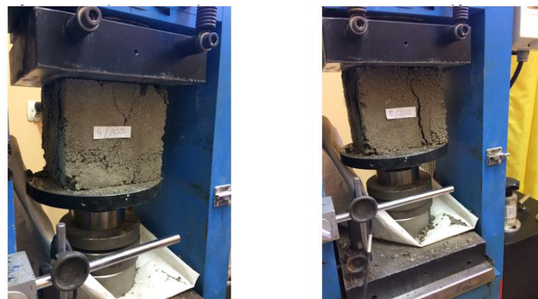
Figure 6. Tests with stress path control—cubic samples [36].
