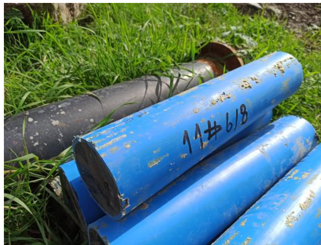
Figure 7. A sample taken from a PVC pipe before delivery to the lab.
