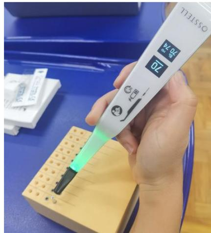
**Figure 6.** Example of the implant stability quotient (ISQ) values assessment through a hand-screwed Smart-Pegs.
