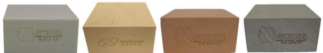
**Figure 3.** Images of polyurethane foam blocks with different densities: from left to right, 10, 20, 30, and 40 pounds per cubic foot (PCF).
