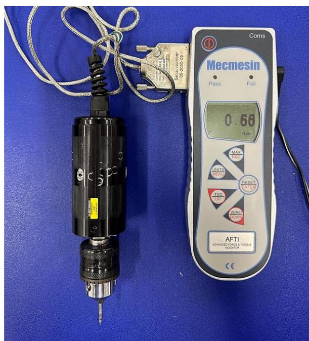
**Figure 5.** Image of the advanced force and torque indicator (AFTI) used to evaluate the insertion torque (IT) and removal torque (RT) values.
