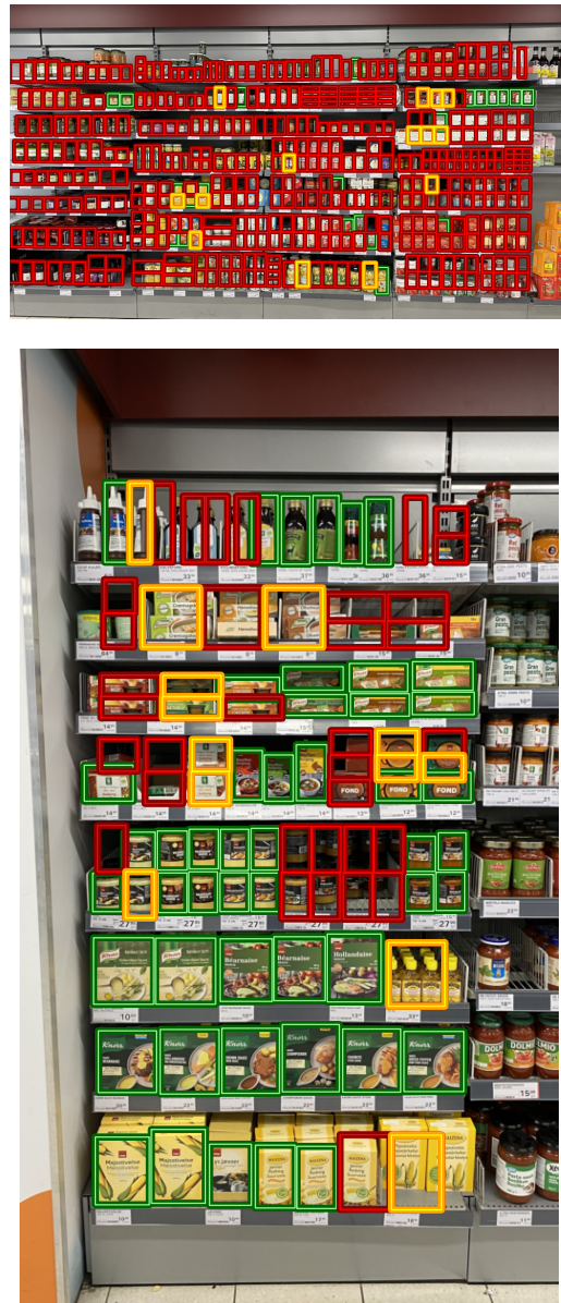
Figure 12. Visualized planogram compliance evaluation performance with internal dataset images 1 ( top ) and 2 ( bottom ). Green boxes signify products originally detected at correct locations, yellow boxes products found after reprojection, and red boxes reprojected boxes that were found not to contain the expected product.
