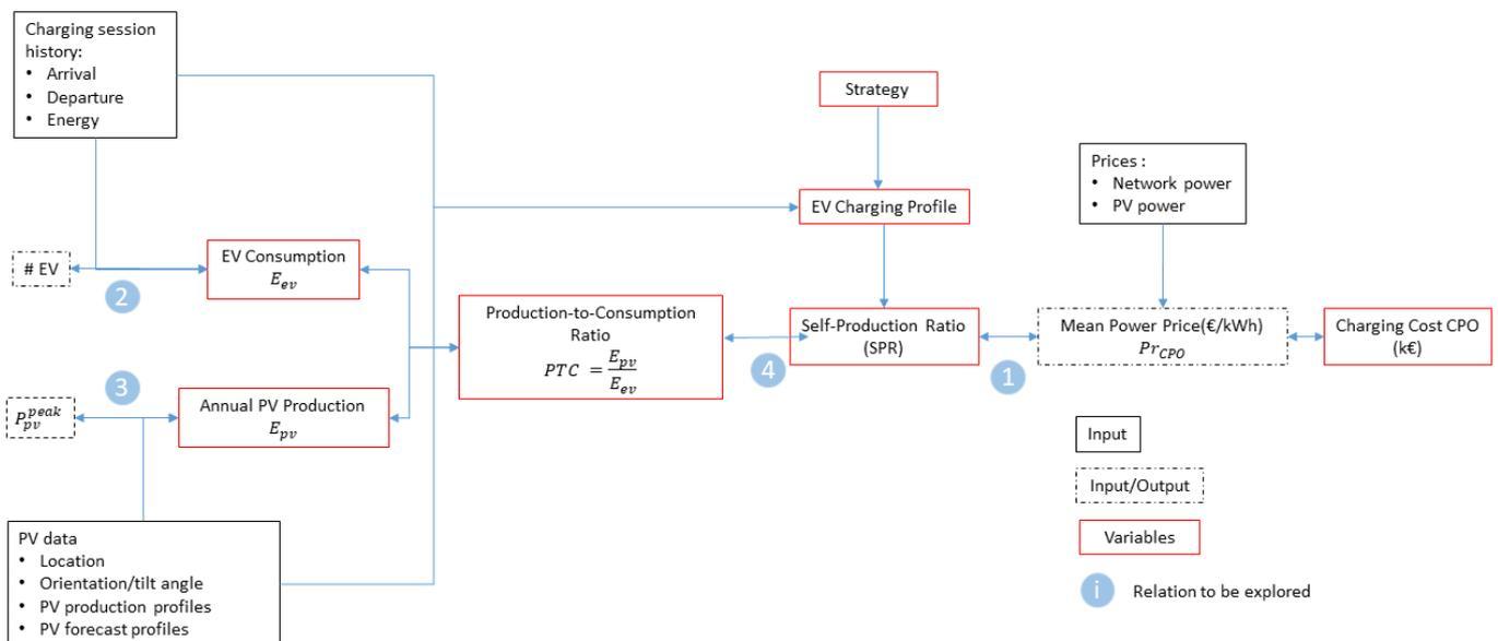
Figure 3. Computational procedure for EV and PV sizing.
