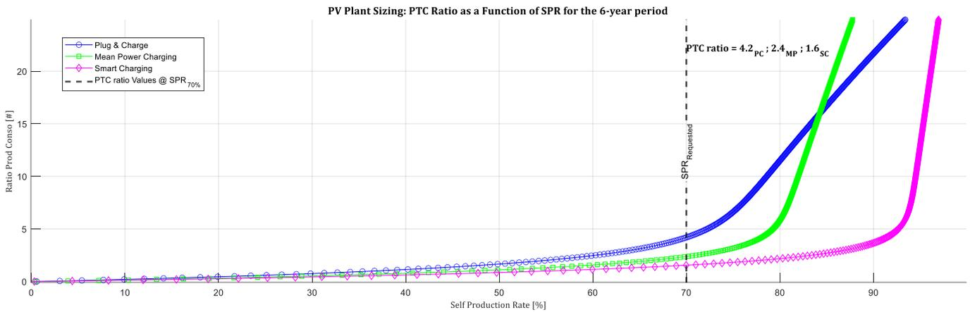
**Figure A2.** Production-to-Consumption (*PTC*) Ratio as a Function of Self Production Rate (*SPR*) for the 6-year period and for the three strategies.
