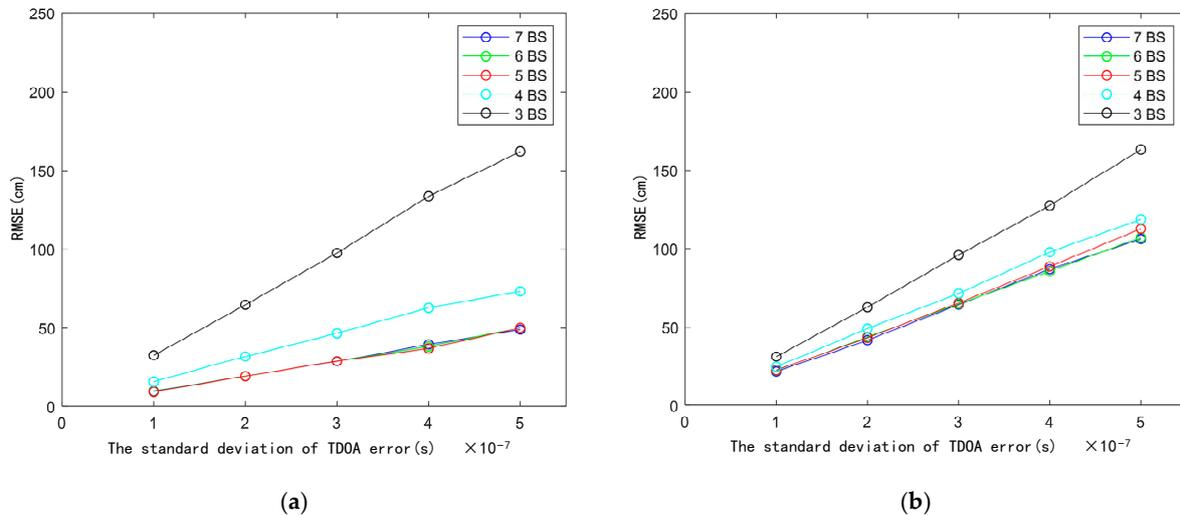
**Figure 3.** Error curves of the Chan algorithm and Taylor algorithm with different numbers of base stations and different TDOA errors. (a) Error curves of the Chan algorithm; (b) error curves of the Taylor algorithm.
