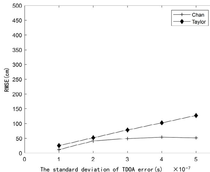
**Figure 4.** Comparison of error curves between the Chan algorithm and Taylor algorithm in four base stations.
