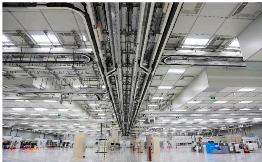
Figure 7. Application scenario of a rail-mounted logistics robot.
