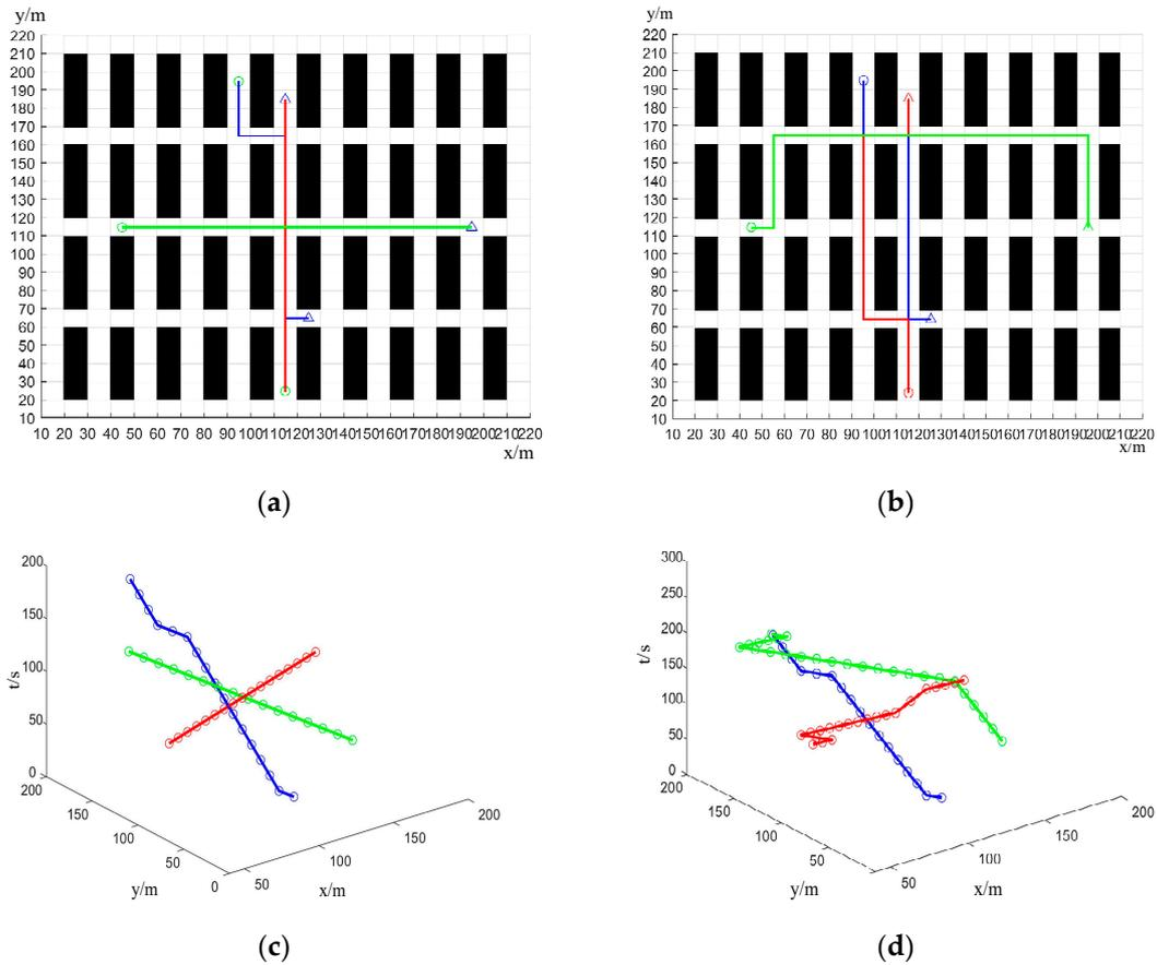
**Figure 9.** (a) The path initially planned by the traditional Dijkstra algorithm. (b) The path is dynamically adjusted by the improved Dijkstra algorithm. (c) The spatio-temporal graph of the planned path before the dynamic adjustment. (d) The spatio-temporal graph of the planned path after the dynamic adjustment. Three lines with different colors represent the planned paths of the three robots, respectively.
