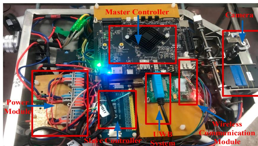
Figure 6. Interior layout of the control box.
