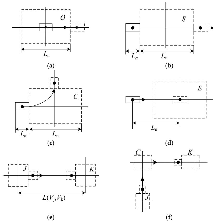
**Figure 2.** The driving situation of the robot in different sites. (a) Driving out of the initial site; (b) going straight through a station; (c) turning to pass a station; (d) pulling into the target station; (e) driving straight into  $V_k$  from  $V_j$ ; (f) turning into  $V_k$  from  $V_j$ .
