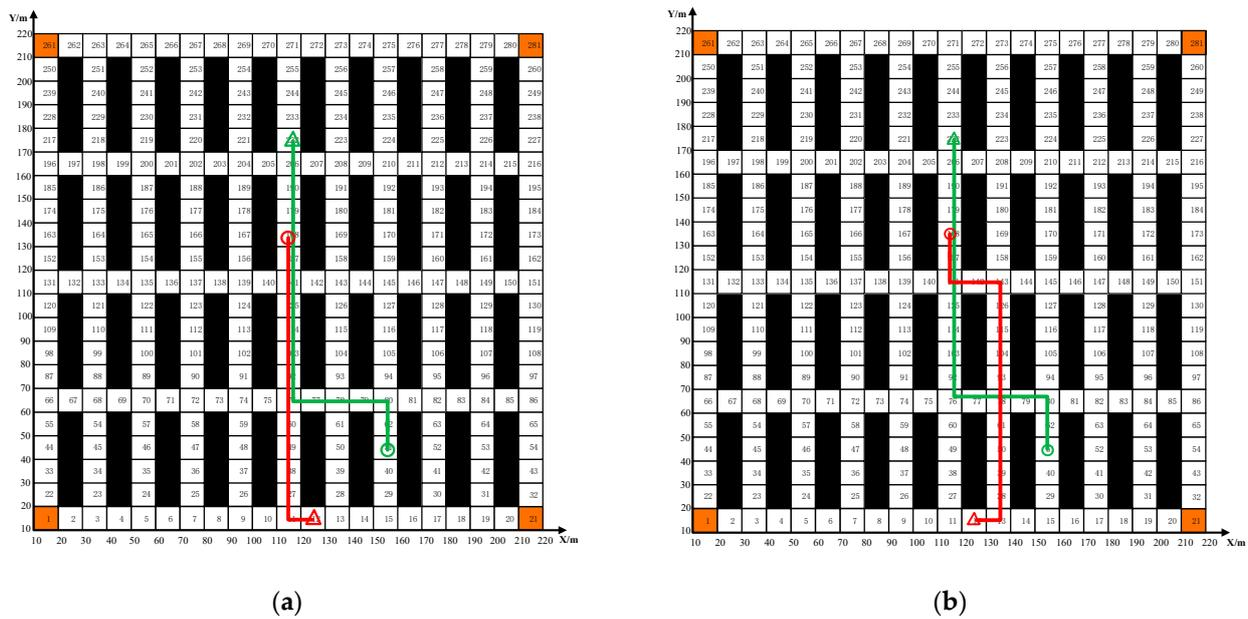
**Figure 10.** (a) Robot route planned before the dynamic adjustment. (b) Robot route planned after the dynamic adjustment. The two lines with different colors stand for the planned paths of the two robots, respectively.
