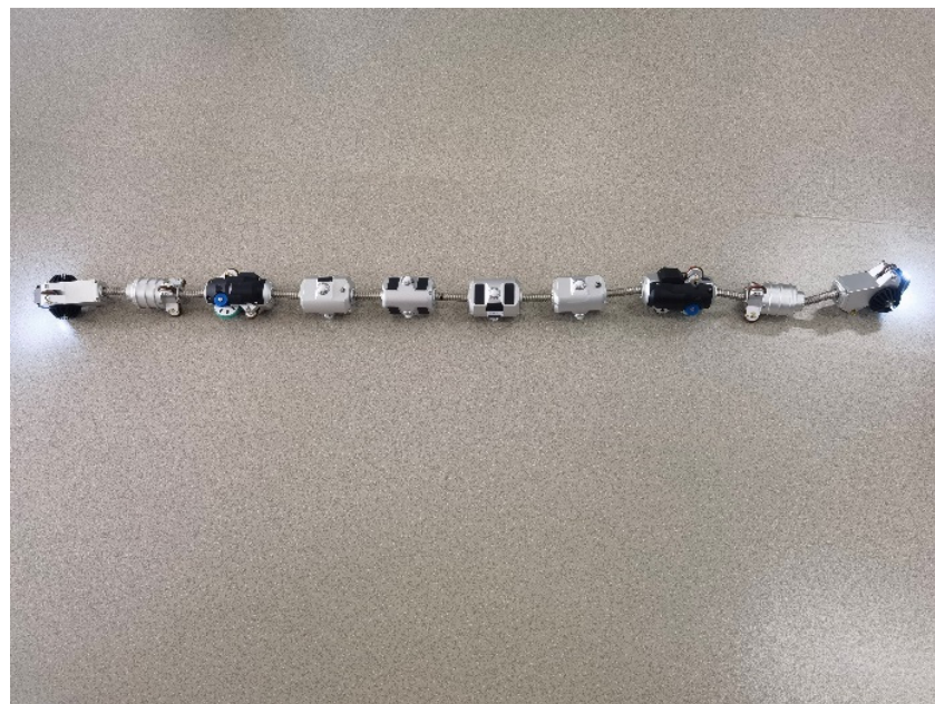
Figure 3. In-pipe inspection robot.
