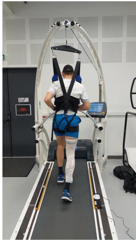
**Figure 1.** Harness Base Body Weight Support Treadmill (Airwalk ap; H/P/Cosmos, Nussdorf, BE, Germany) with (Optojump; Microgate, Bolzano, Italy).
