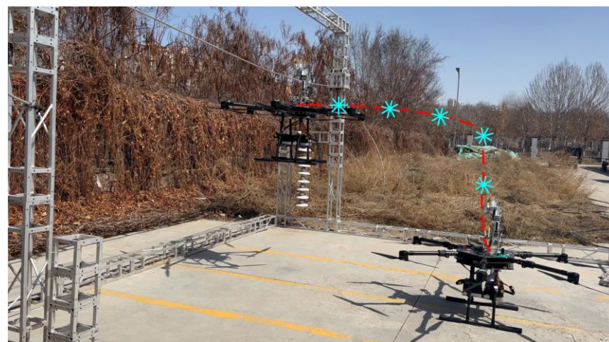
Figure 17. The fast landing stage of the FPLIR.
