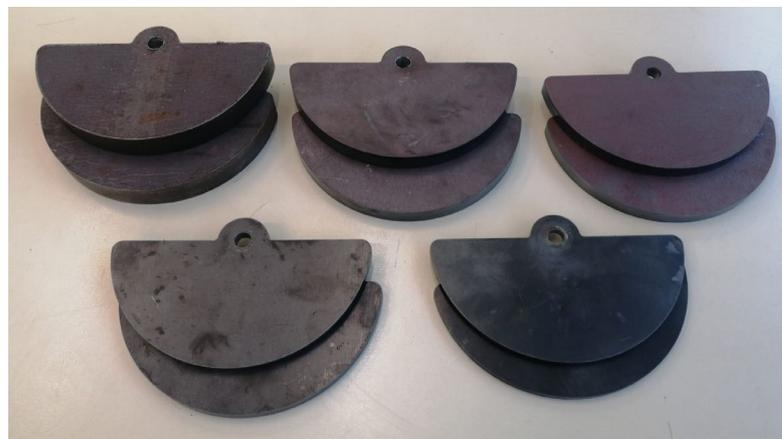
**Figure 7.** Eccentric bodies with different masses (cut from steel sheets with different thicknesses).
