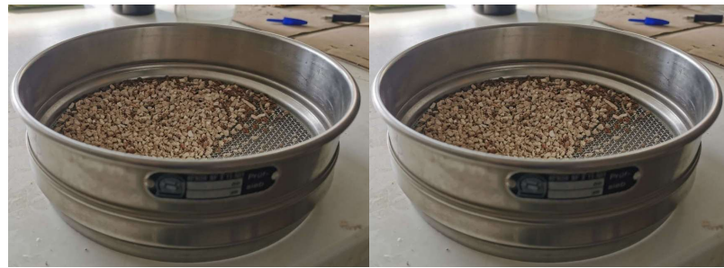
Figure 22. Sieves showing angular and subangular gravels with a diameter > 8 mm and the coarse sand of the first semester sample.
