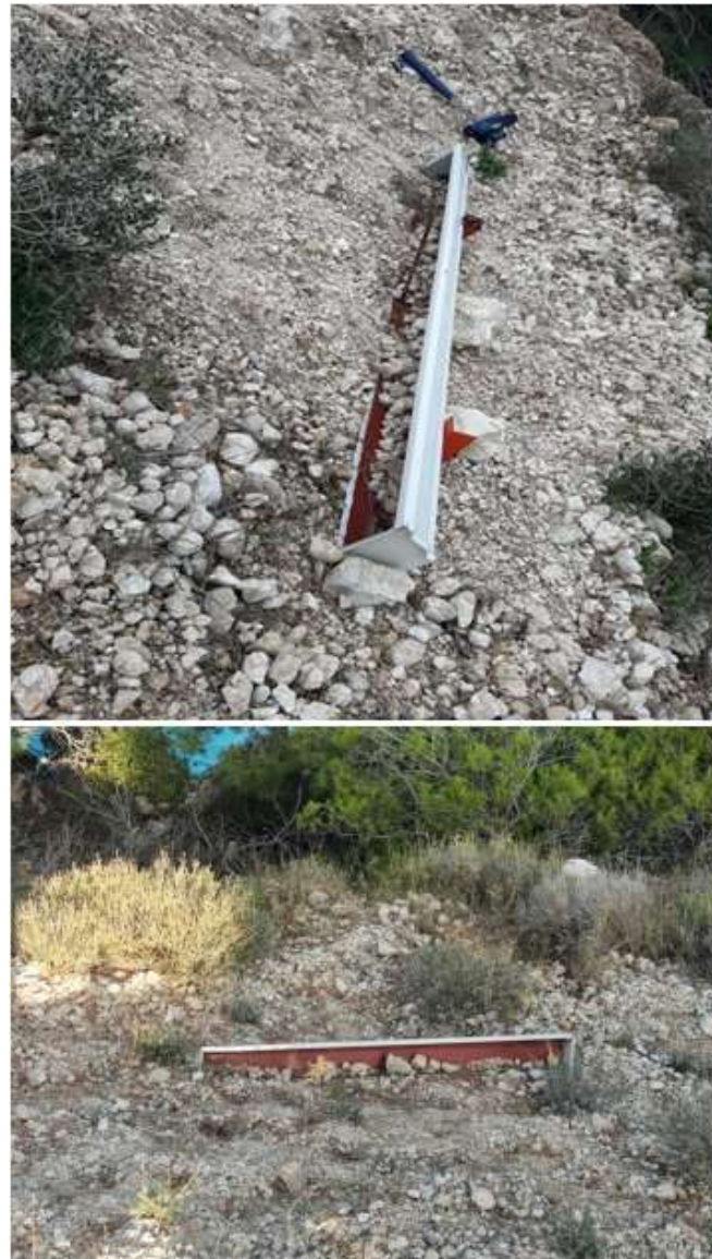
Figure 4. The sediment trap that was placed on the overhanging cliff located in Egremni beach.
